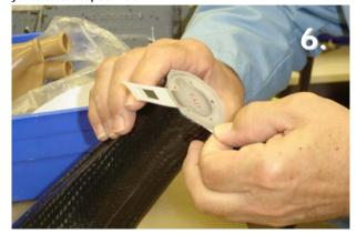
The Template is Translucent and the exact size of the face of the Lamination Ring. Cut the Template out and glue or tape it to the Lamination Ring. Be sure and line up the boltholes exactly. Fold the Slot Locator down the side of the socket and glue or tape it in place.
