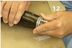
The Rotator Lever Switch should then pop up through the Rotation Lever Slot.
