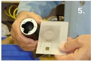
The Rotation Switch Slot Template is provided. This Template will help you to locate slot placement.
