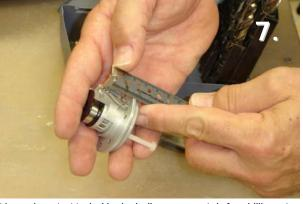
It is very important to double-check all measurements before drilling out the Rotation Lever Slot.
