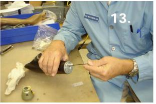
Now you can replace all 4 Counter Sunk Mounting screws and the 1 Rotation Stop Socket Head Cap Screw.
